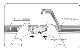
4 Screw the end connector plate with the A top surface and B top surface tightly.
