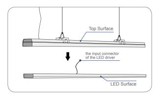
2 Split the LED surface and the top surface, then take off the input connector of the LED driver.
