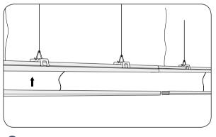
6 Raise the LED surface to a proper high, connect AC input wires with the LED driver, install the LED surface back together with the top surface in the help of other people, install the end caps at each side, interconnection works.
