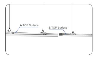
3 Take off the end caps at each side of the new fixture, follow the step2, split it's LED surface and top surface, completely up the top surface of the new fixture, adjust the position, making sure the two fixture line closely.
