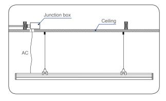
Find a suit hanging position, hand up the lamps, plug in then complete the installation;
