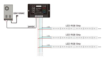
[Attn]: Power repeater can be added if connect to more LEDs, please refer to the manual of power repeater for the specific connection method.
