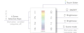
\* When the touch panel is off, Long press  $\bigcirc$  to turn on/off the buzzer When the touch panel is on "Long press  $\overset{\smile}{\bigcirc}$  to match code.
